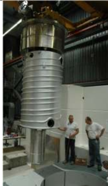
Pb/Zr spallation target (about 8 neutrons per proton)
